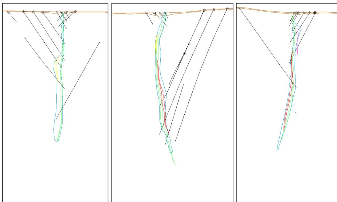
Figure 9.24 Profiles 3 (left), 14 (middle) and 19 (right). Images show drillholes used in the estimation and magnetite skarn (blue outline), D1 (green outline), D2 (red outline) and d3 (yellow outline). Also, topography and base of the overburden is shown in brown.
