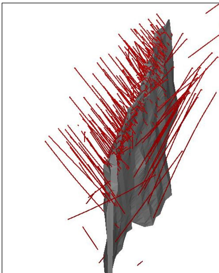
*Figure 7.2 3D inclined perspective view looking north showing drill holes at D Zone and the mineralised magnetite skarn unit*
