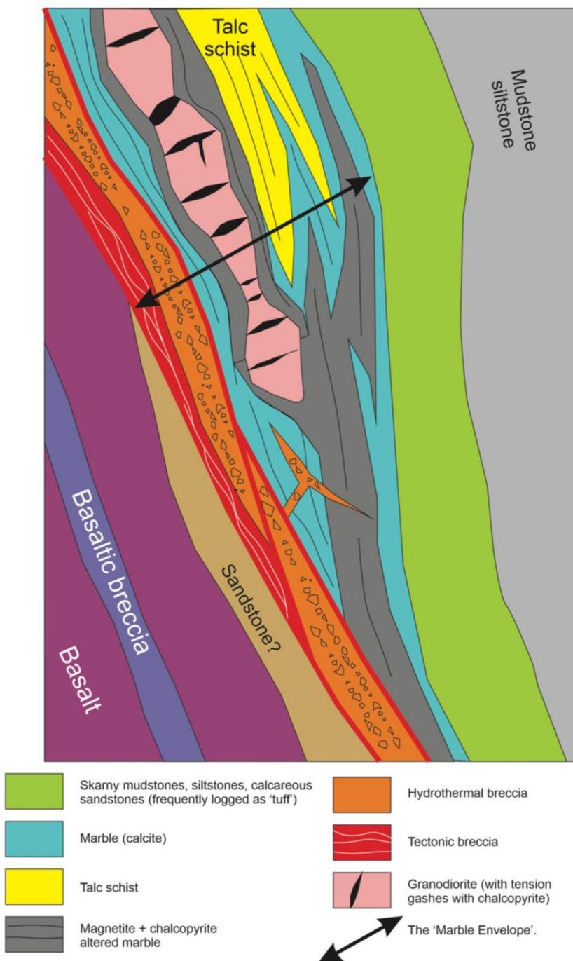
Figure 8.3. Schematic west to East section on the D lens. By Pratt, 2020. Note also the Cu-rich vein style of mineralization emplaced in tension gashes within competent units (Fig.8.6)
