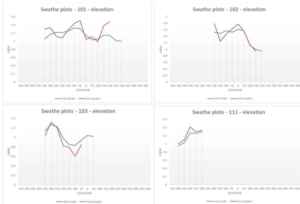
Figure 9.26. Swath plots Cu(%) vs elevations showing sample grades in red and model grades in blue.
