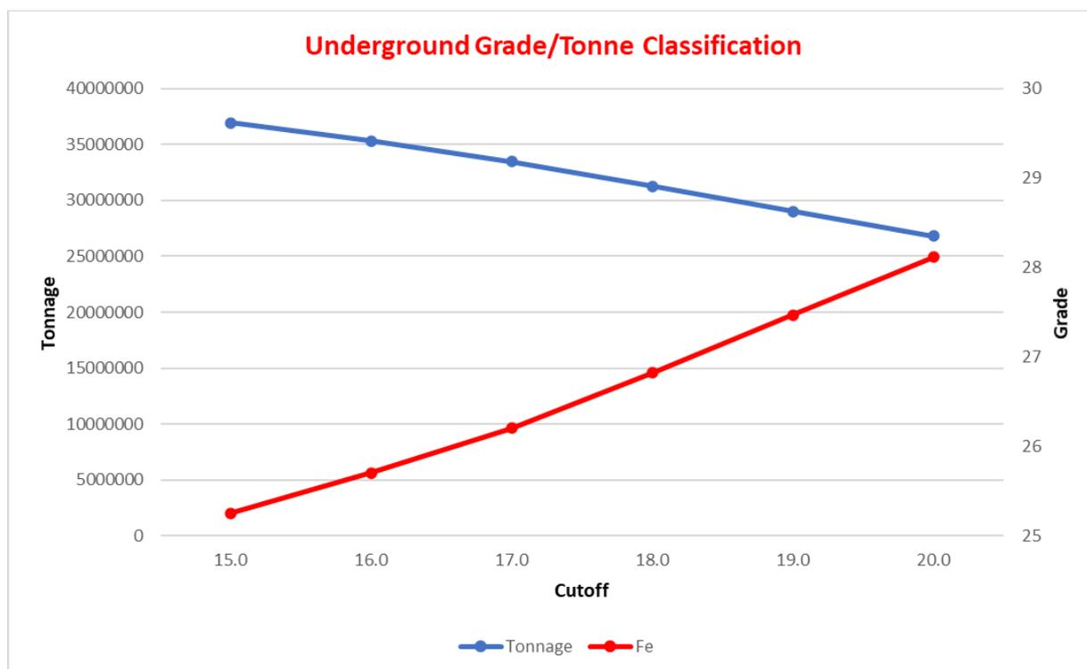
Figure 9.35. Grade tonnage curve of underground mineral resources of all fe domains.
