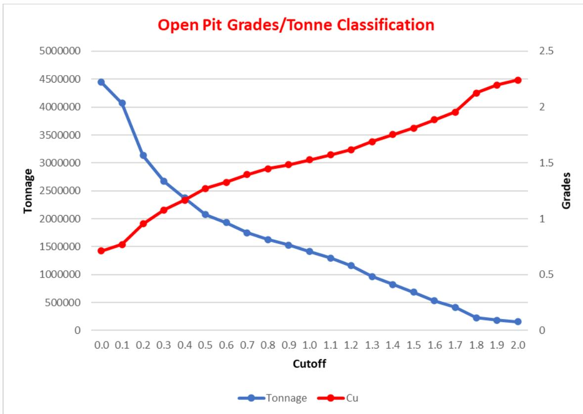
Figure 9.31. Grade tonnage curve of open pit mineral resources of all cu domains.
