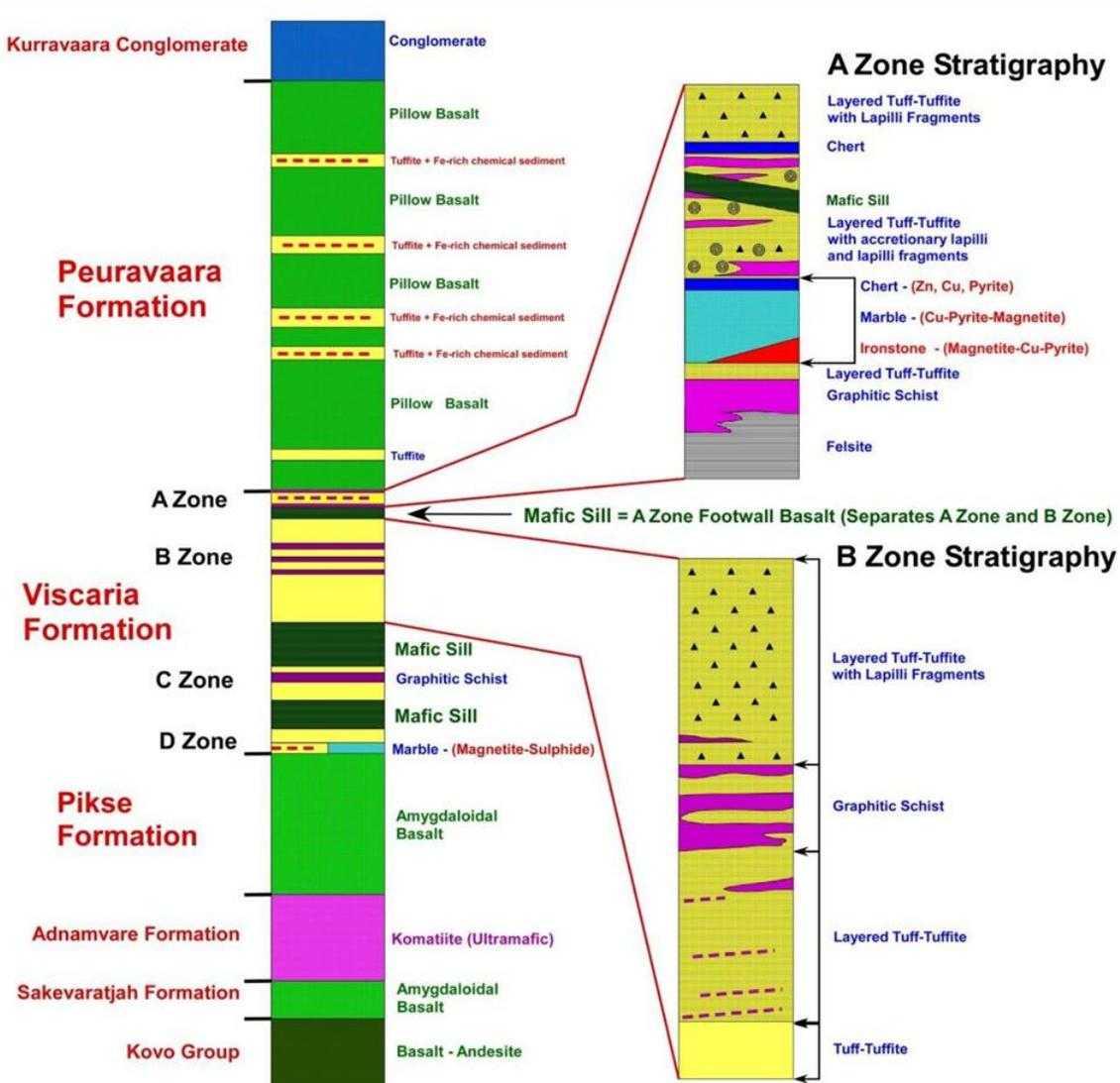
Figure 8.1. Detailed stratigraphic column for the Viscaria area. A, B and D ore horizons are hosted within the sedimentary rich part of the sequence.
