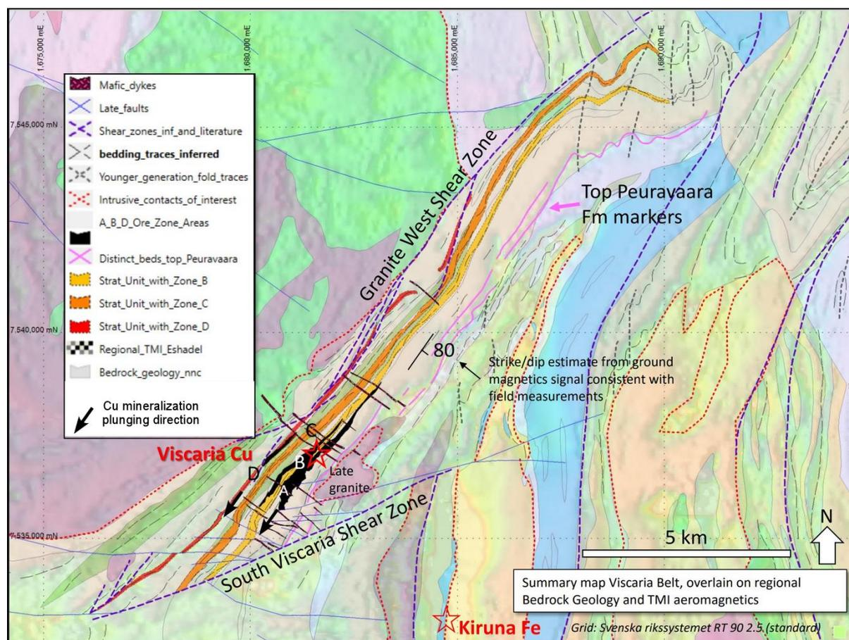
Figure 8.2. The South Viscaria shear zone controls the south extension of the ore hosting lithologies. Drilling intersections and structural interpretations Pratt, 2020 for extension of the D ore lenses at depth indicates partly an structural control on the steeply dipping plunge of higher Cu grades and increased mineralized thickness towards the South West.
