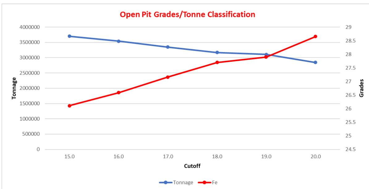
Figure 9.34. Grade tonnage curve of open pit mineral resources of all fe domains.
