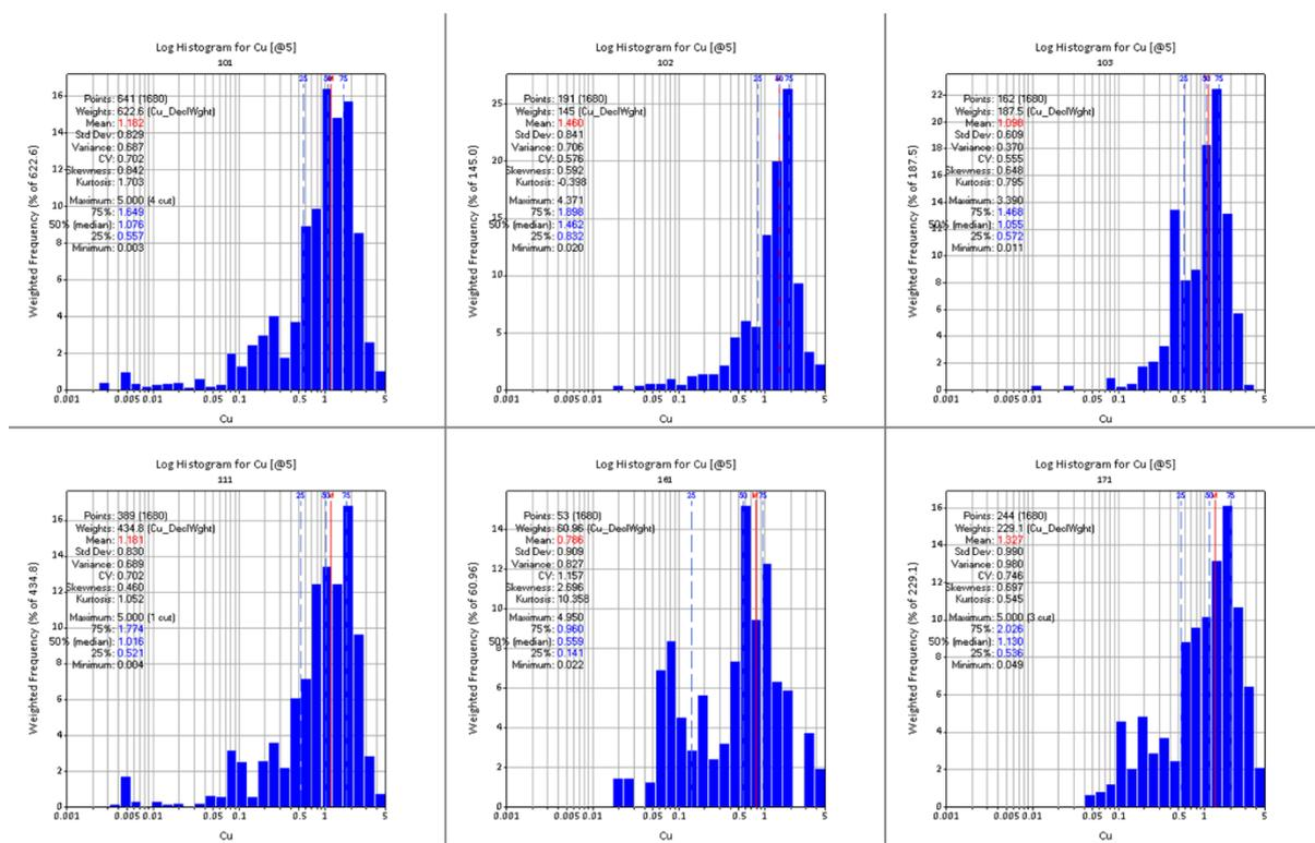
Figure 9.9. Copper grade population in the log histogram. X-axis shows copper grade and y axis shows frequency. Domains from left to right are top row 101, 102, 103 and bottom row 111, 161, 171.
