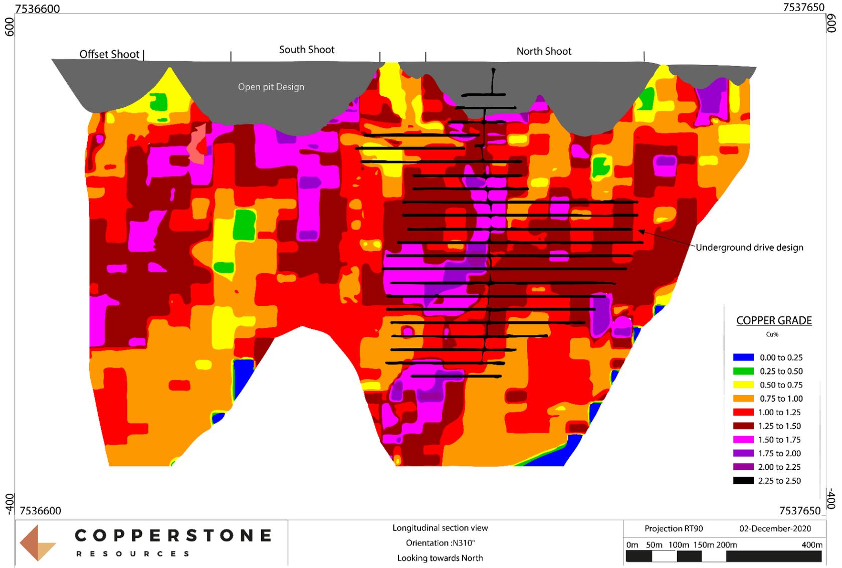
Figure 9.18. SW-NE longitudinal section over D zone showing estimated copper grade in the block model with 2016 scoping study mine design shapes
