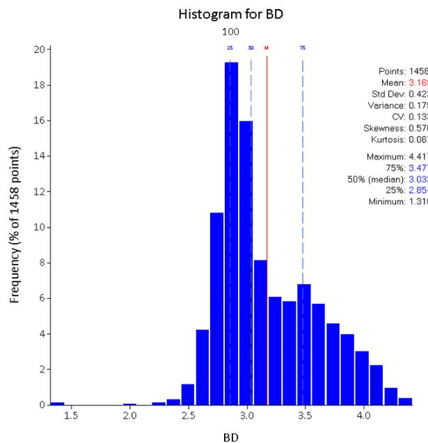
Figure 9.22. Bulk density of the magnetite skarn of Viscaria D zone.
