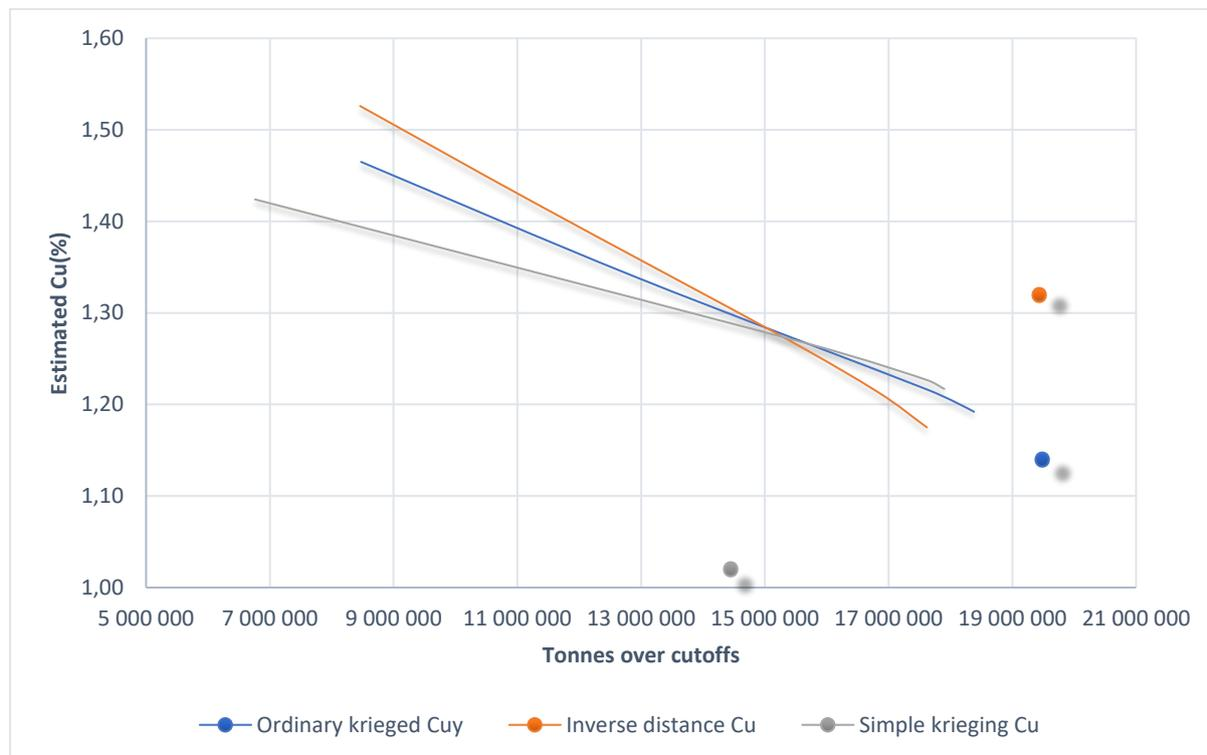
Figure 9.27. Grade tonnage curve comparison of three different estimation methods
