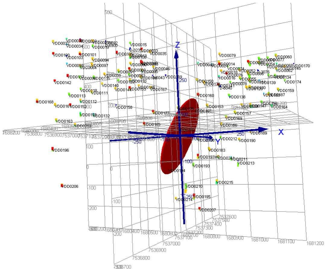
Figure 9.12 Image shows variogram ellipsoid for Cu and composite sample data in the domain 101.
