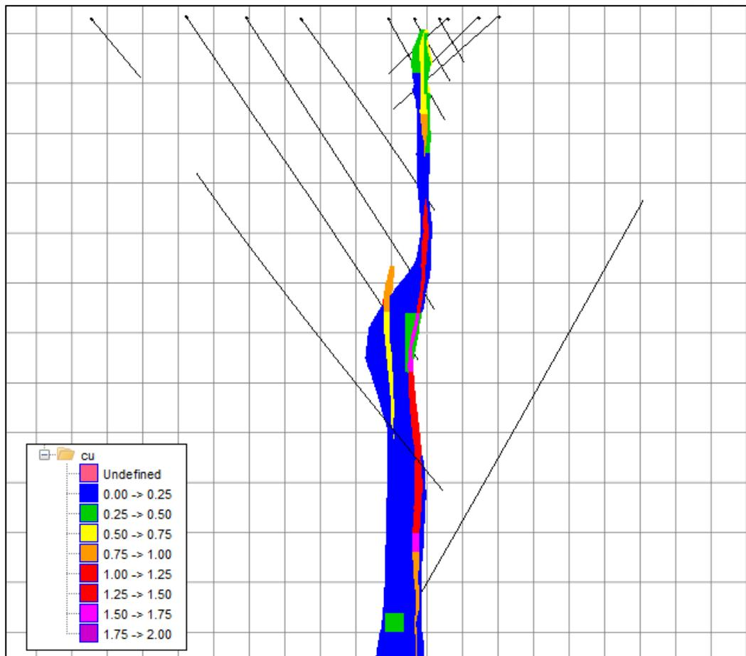
Figure 9.17. Oblique cross section 3 which locates in the middle of the D zone south shoot. Drillholes are shown in the black traces and block model as copper grade-coloured volumes. The grid is 50m x 50m and the deepest drillhole is Copperstone drilled hole VDD0206.
