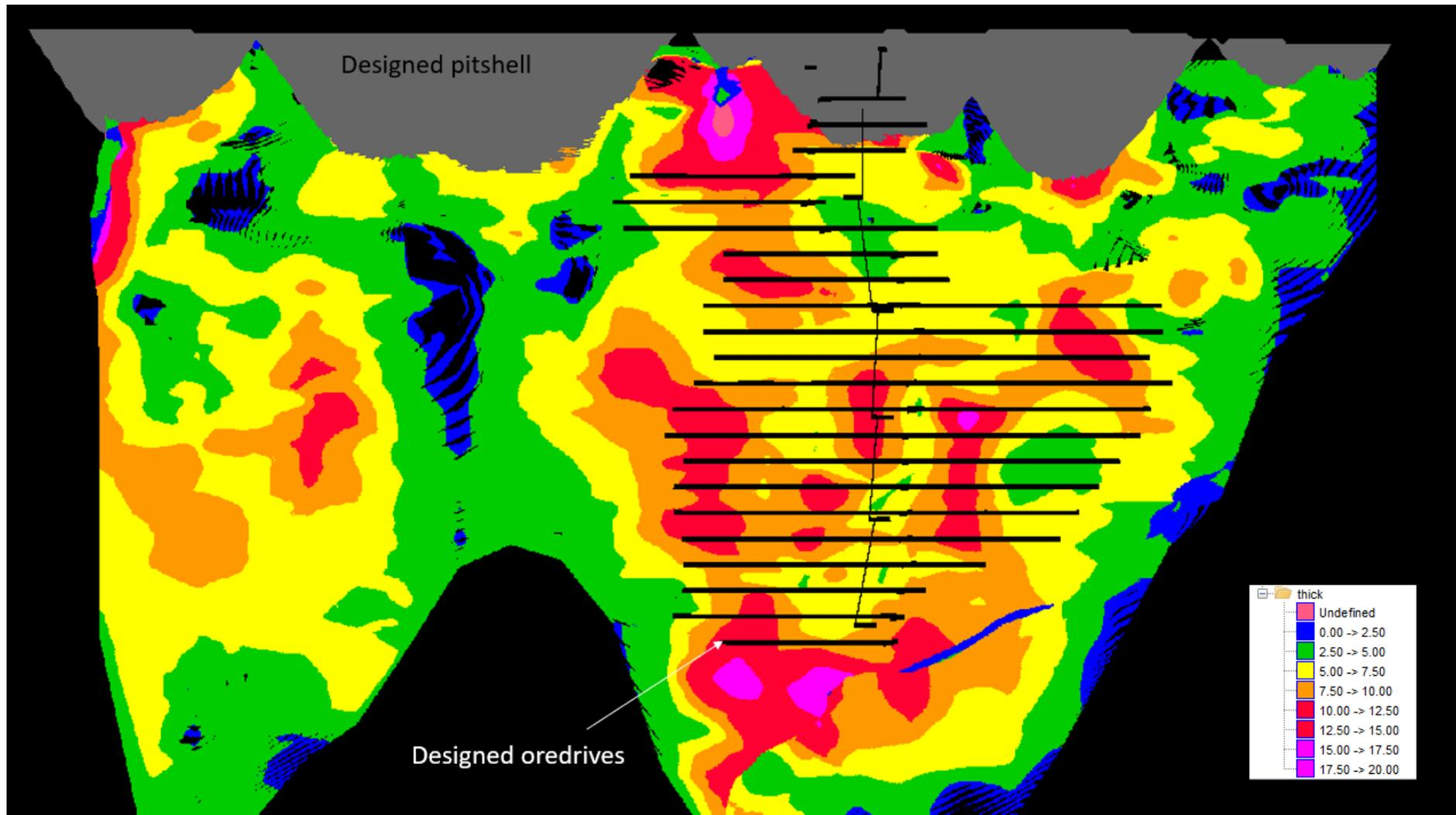
Figure 9.19 SW-NE longitudinal section with thickness variations in the D1 mineralisation with 2016 scoping study's mine design shapes.
