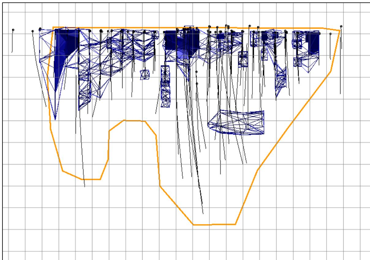
*Figure 9.2. Longitudinal NE-SW image over Viscaria D zone showing location of the oxidation zones. Blue polygons show Complete Oxidation and blue triangles show partial oxidation. The Mineral Resource outline is shown in orange line and a 100mx100m grid is shown for scale.*
