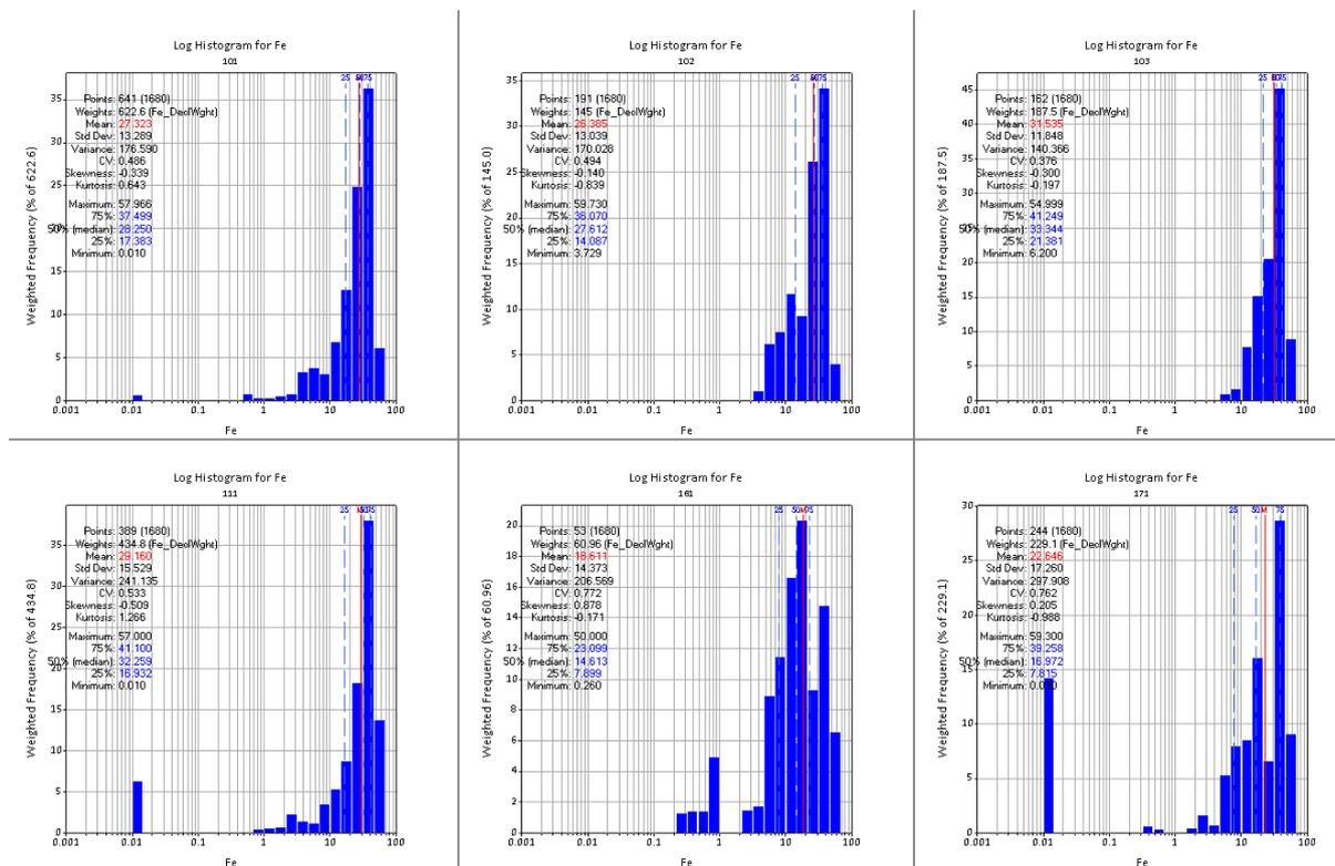
Figure 9.10. Iron grade population in the log histogram. X-axis shows iron grade and y axis shows frequency. Domains from left to right are top row 101, 102, 103 and bottom row 111, 161, 171.
