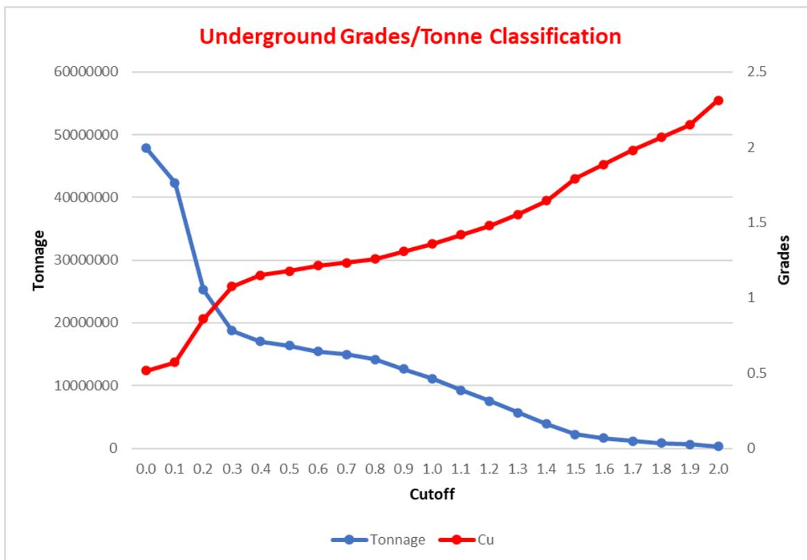
Figure 9.32. Grade tonnage curve of underground mineral resources of all cu domains.
