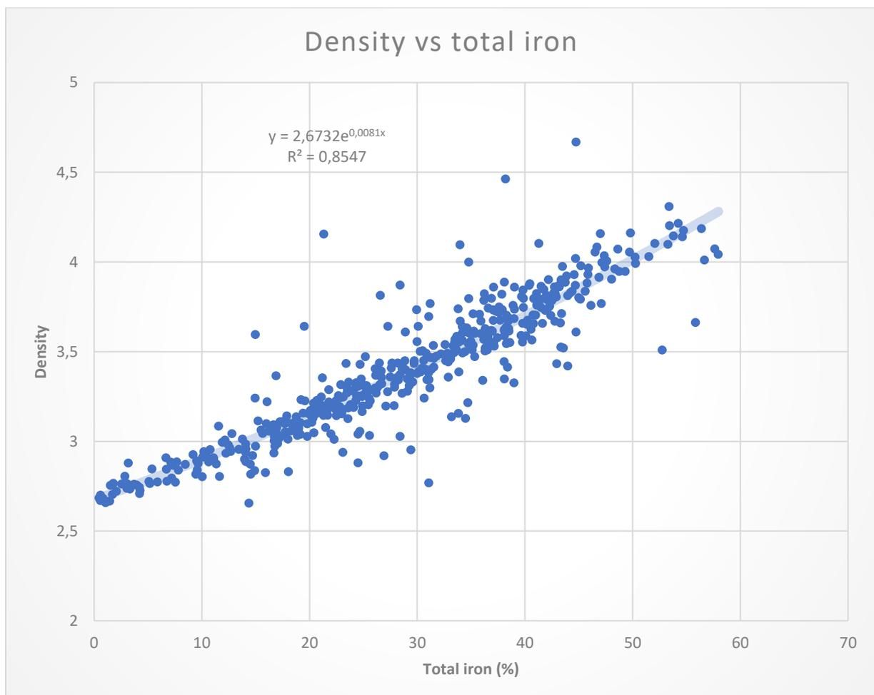
Figure 9.23 Scatter plot showing correlation between total iron content and density of the rock. Correlation of density to iron is excellent, allowing polynomial fitting as a comparative density calculation method.
