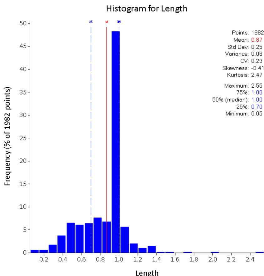
Figure 9.5. Histogram of sample lengths of mineralised domain before compositing.
