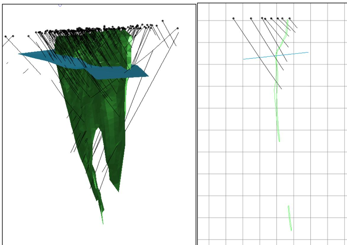
Figure 9.1. Left (3D image of the D1 main mineralisation in green and subdomain boundary in blue. Subdomain boundary shows distinct change of the orientation of mineralisation. Right. Cross sectional view of the D1 main mineralisation (green) subdomain boundary (blue). Grid shown is 100m x 100m.
