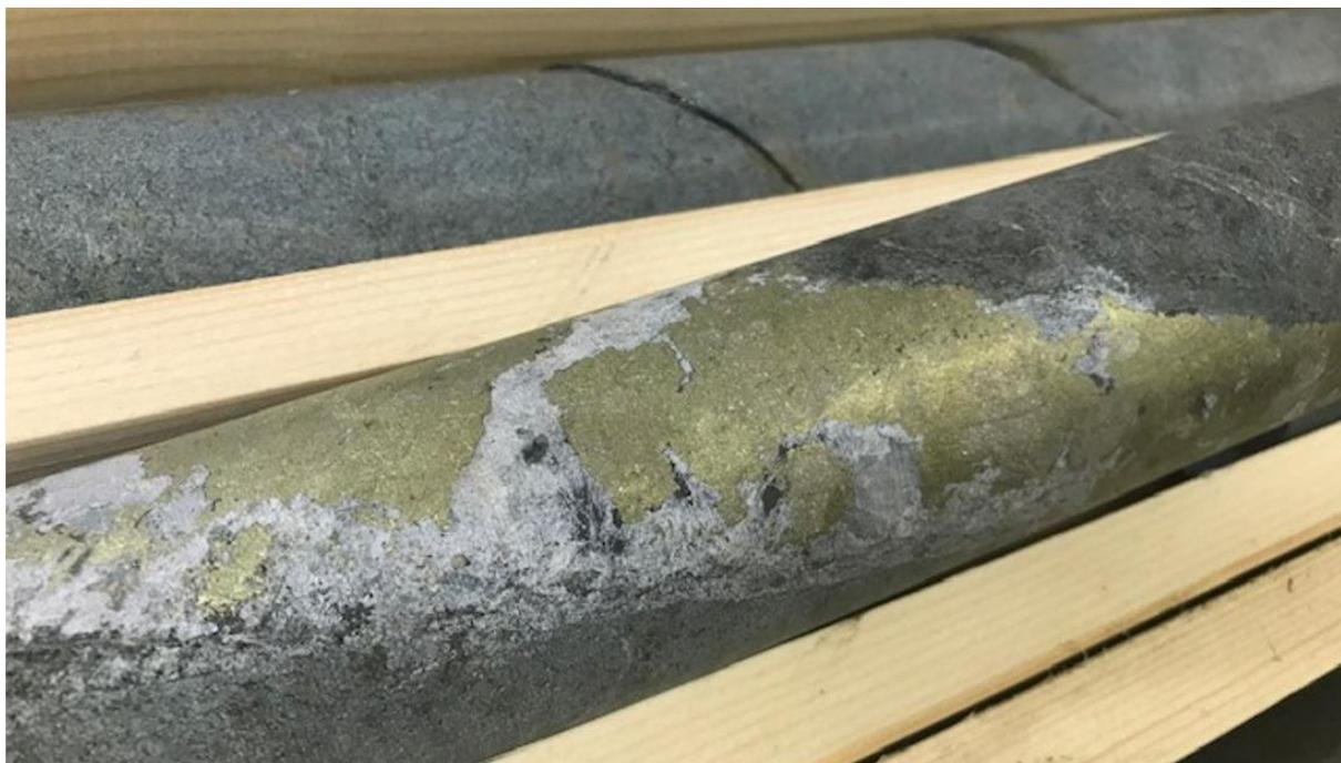
Figure 8.6. Chalcopyrite carbonate vein cuts through coherent intrusive units located on the hanging wall side of the D lens. The epigenetic origin of this type of Cu mineralization correspond to a group of reactivated structures and dikes orthogonal to the sedimentary trend that might be associated with tensional dislocation and sulphide remobilization along mechanically competent units.
