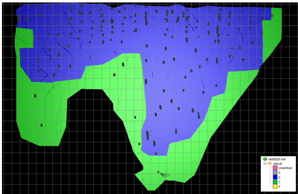
Figure 9.29. Longitudinal view showing resource classification and composites in the estimation. Blue colour shows indicated resources and green colour shows inferred resources. Black dots are sample composites used in the estimation.
