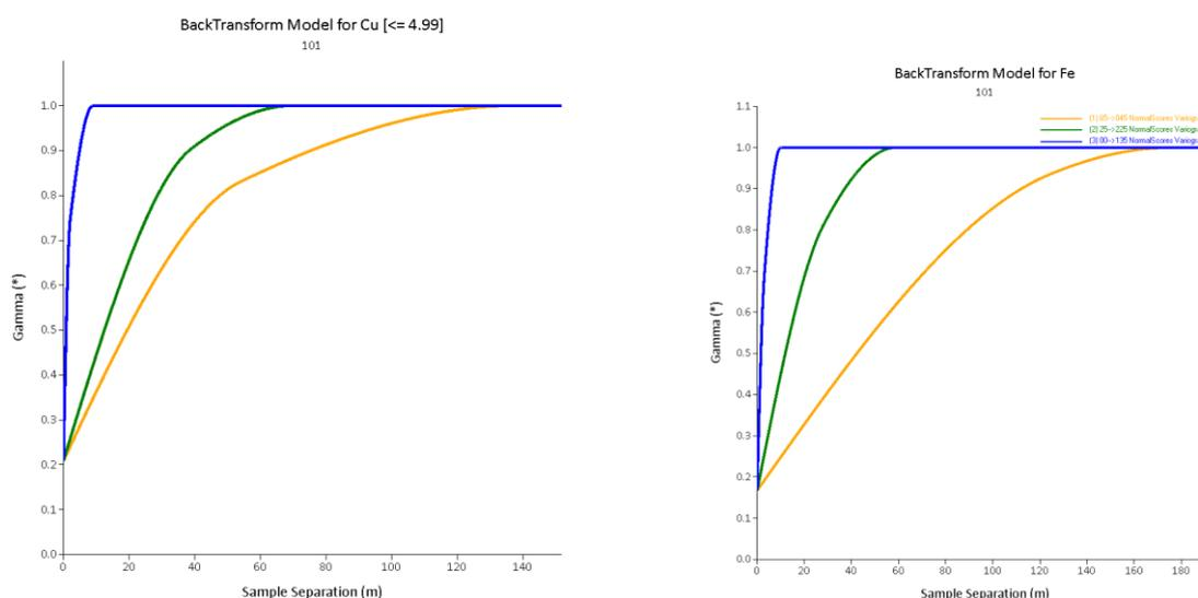
Figure 9.15. Modelled directional variogram for Cu (left) and Fe (right) with backtransformation applied
