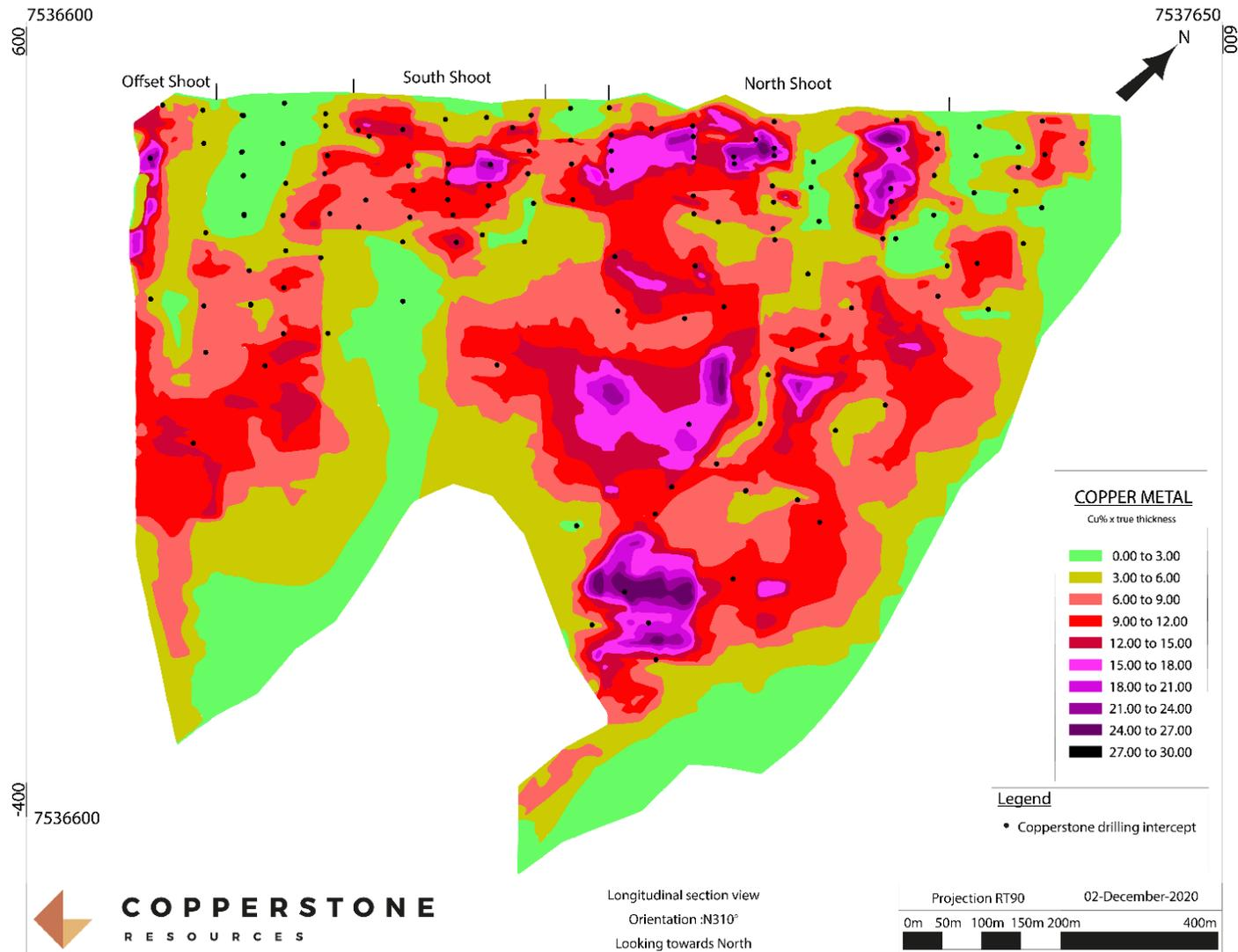
Figure 9.20 SW-NE longitudinal section with copper metal in the D1 mineralisation. Copper metal is calculated using true thickness of mineralisation calculated from the block model and multiplied by estimated copper grade
