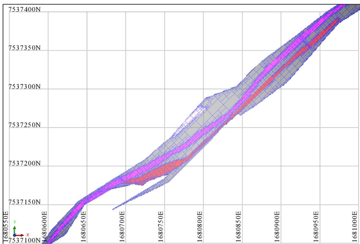
Figure 9.16. Plan view of the Viscaria D zone at elevation 0mRL which is about 500 metres below surface. Orientation of the rotated block model vs magnetite skarn shape (yellowish gray), D1 mineralisation (purple) and D2 mineralisation (red).
