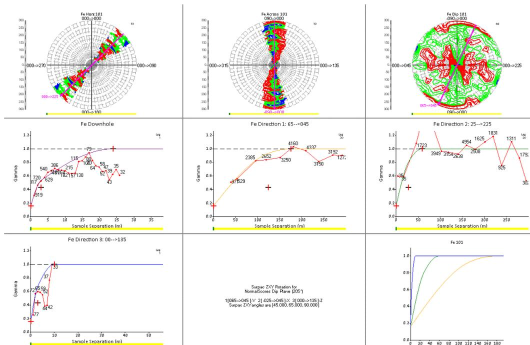
Figure 9.14. Variography analysis for iron in domain 101. Images are from left to right: top row. Variance images in the strike plane (left), dip plane (middle) and plunge plane (right). Center. Directional variograms major direction (left), semi-major direction (center) and minor direction (right). Bottom. True downhole variogram (left), modelled direction definition (center) and modelled variograms in normal score space (right).
