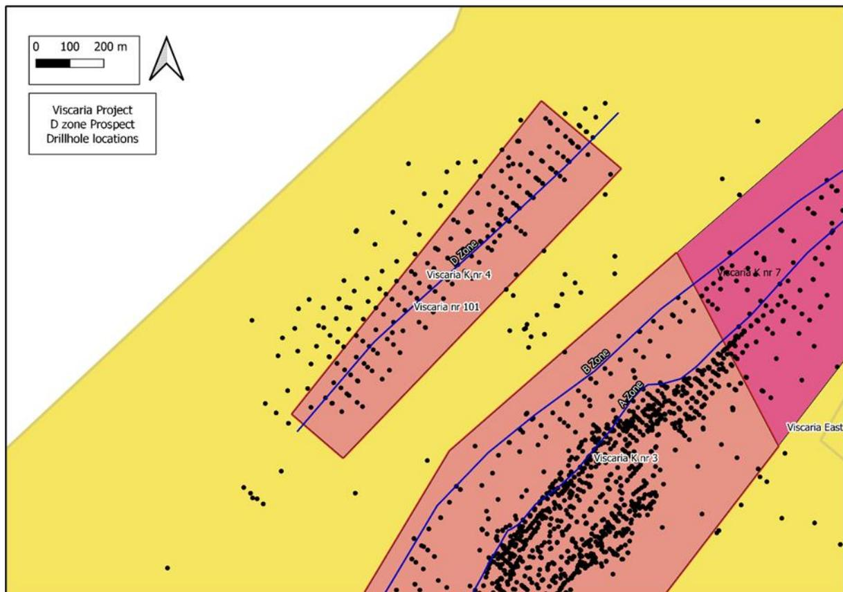
Figure 7.1 D Zone drill hole locations
