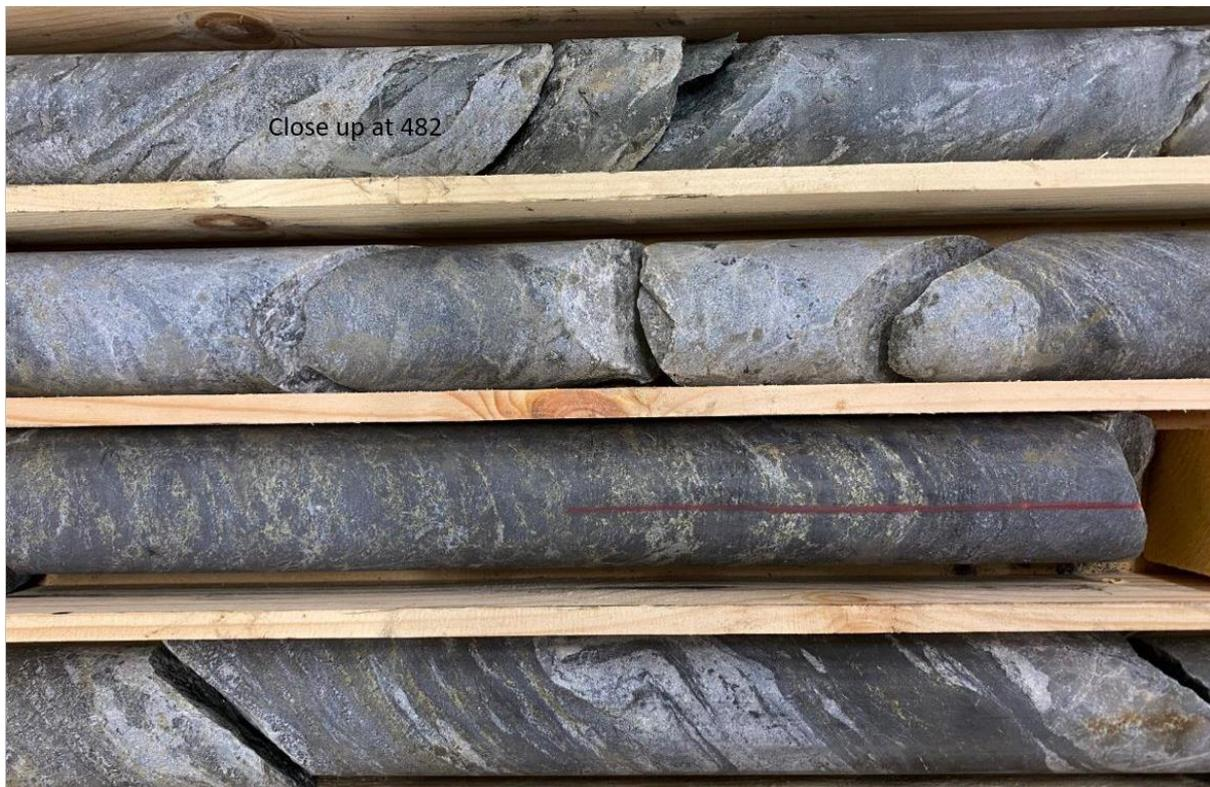
Figure 8.5. Drillhole VDD0242 @482m. Roughly banded Cu sulphide mineralization (chalcopyrite) replacing along margins of magnetite zones and disseminated carbonates in the D ore.
