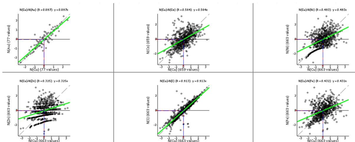
Figure 9.11 Bivariate scatter graphs in normal score scale to visualise correlation of element pairs. Data is shown for domain 101 and graphs are from left to right and top to bottom – Cu-Au, Cu-Co, Cu-Ni, Cu-Zn, Cu-S and Cu-Fe.
