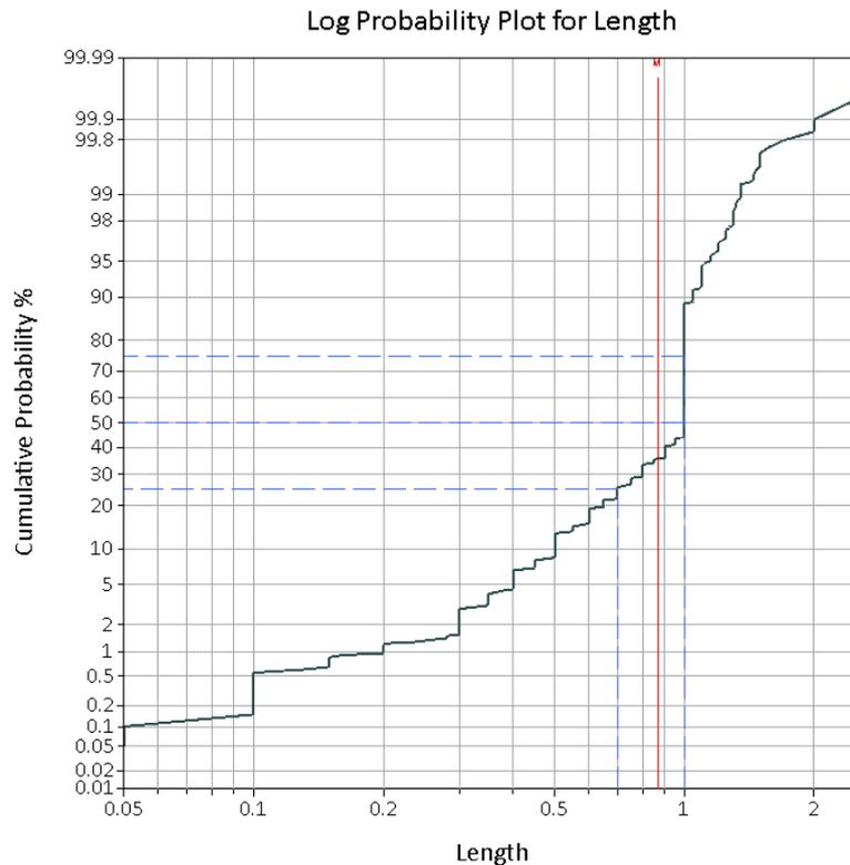
Figure 9.6. Log-probability plot of sample lengths of mineralised domain before compositing.
