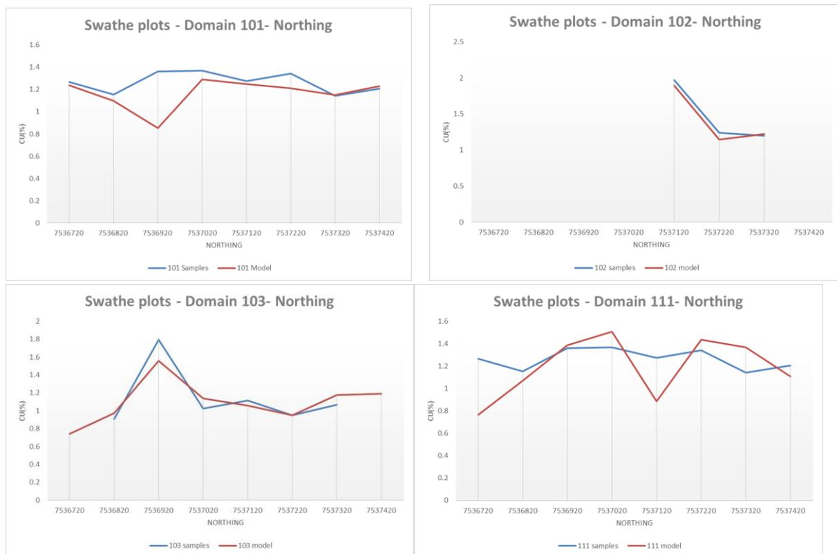
Figure 9.25. Swathe plots Cu(%) vs northing showing sample grades in blue and model grades in red.
