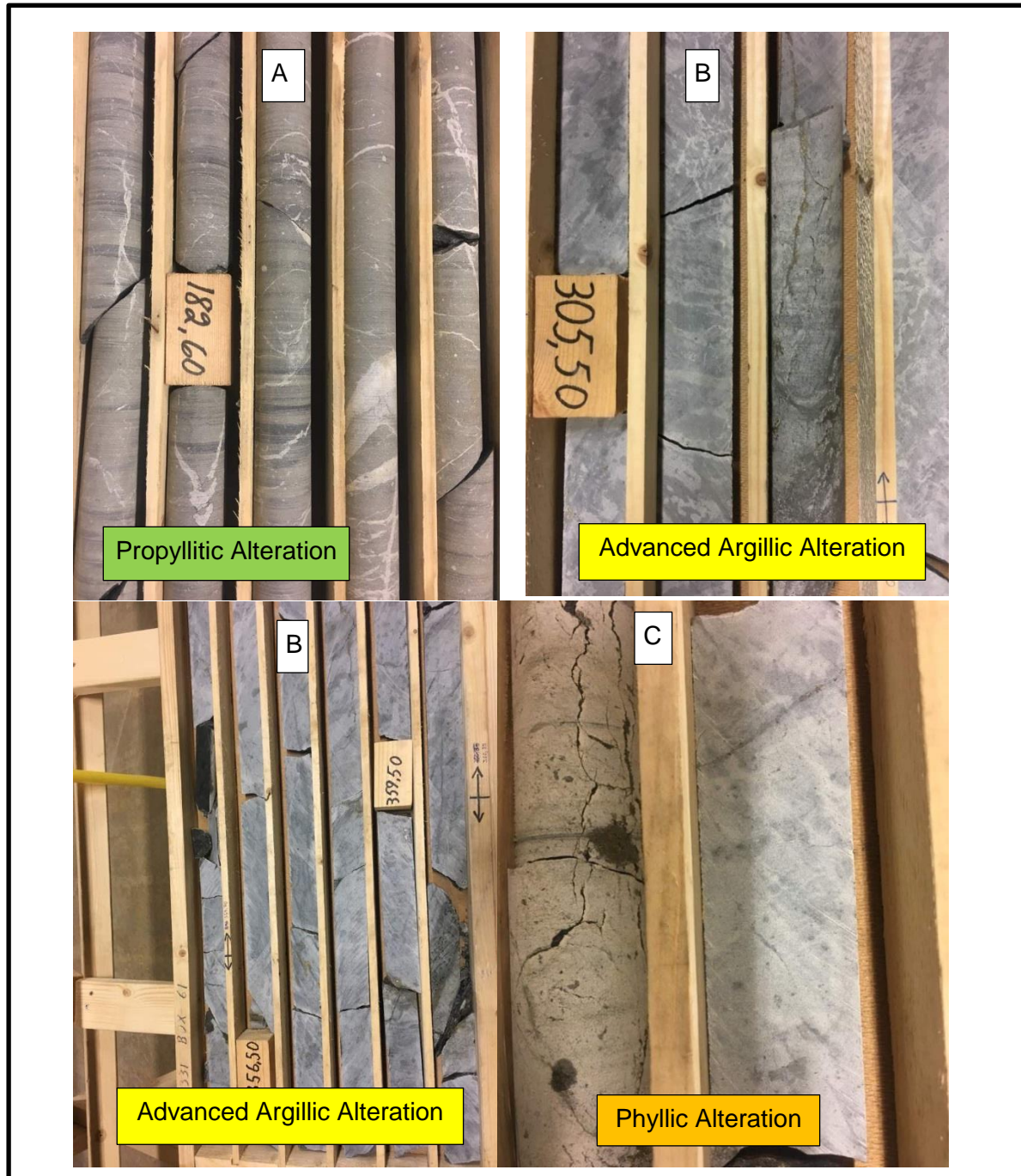
Figure 17: Types of alteration drilled in COS07334.
