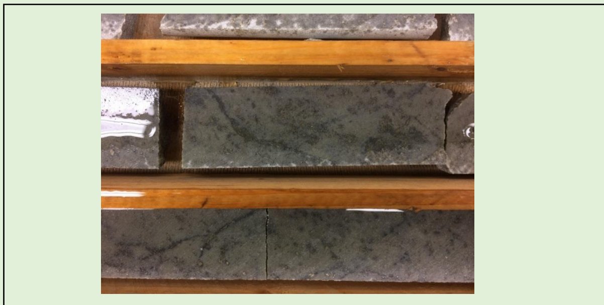
Figure 2: Photo of the phyllic alteration showing the typical yellow colour and “spotty” pyrite
