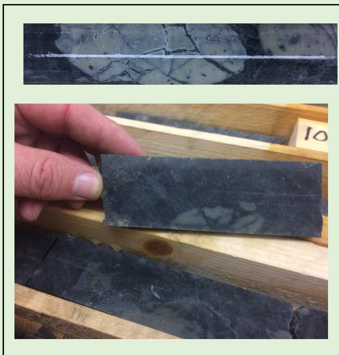
Figure 7: The polymictic clasts which have themselves undergone a degree of brecciation subsequent to being emplaced.
