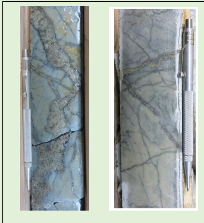
Figure 4: Crackle breccia – ruptures and cracks filled with pyrite in a highly siliceous matrix.
